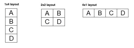
**IMPORTANT** Individual outputs cannot be assigned a position, therefore monitors must be connected to the Mura DVW device in the correct order from left to right (A to D).
