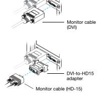
If your monitor cable has an HD-15 connector, use the DVI-to-HD15 adapter included with your Matrox product to connect your monitor to the secondary connector.
