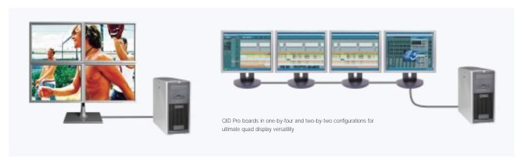
The QID Pro can also be paired with the Matrox Advanced Synchronization Module (ASM) in order to Genlock and Framelock footage being displayed across multiple screens. Taking this one step further, the Matrox ASM can also synchronize multiple systems equipped with QID Pro graphics cards, providing truly astounding multi-monitor real estate for a visually impacting set-up.
