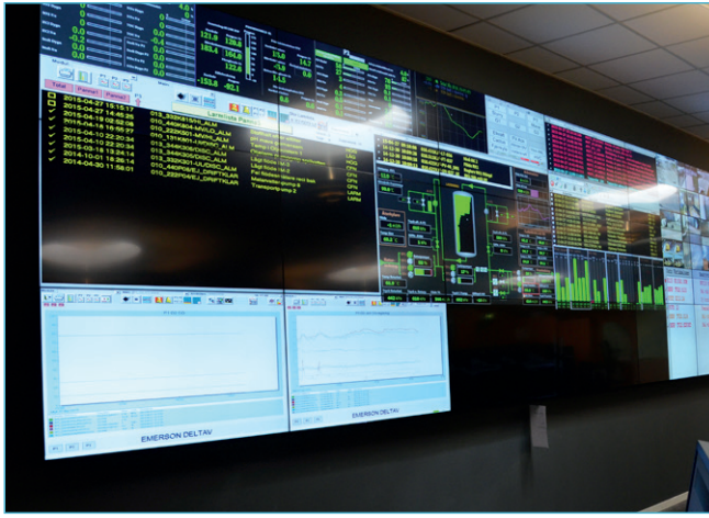
Mura MPX cards capture and display a variety of inputs on the video wall, including content streams and data pertaining to the many sites monitored by the plant's control room employees.
