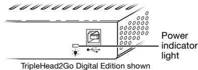
**Solution** Make sure your power supply cable or USB cable are properly connected. For more information, see [“Connection setup – TripleHead2Go Analog Edition”](#), page 4 or [“Connection setup – TripleHead2Go Digital Edition”](#), page 7.
