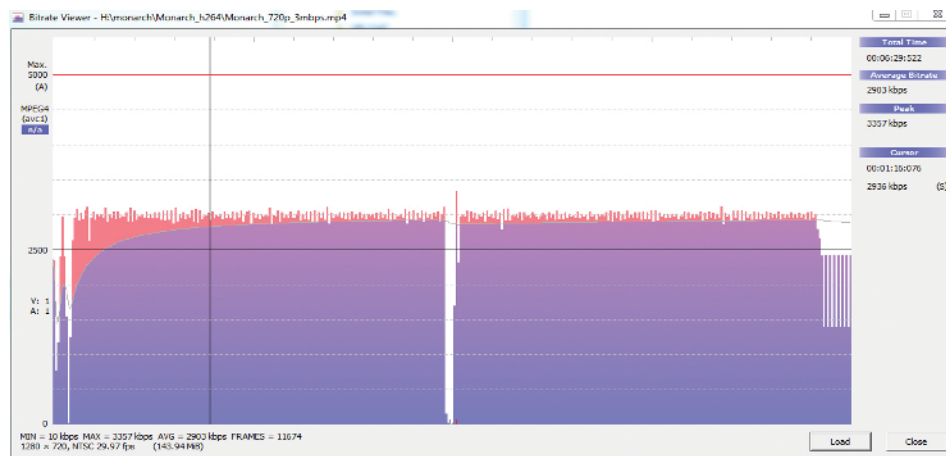
Figure 3. Bitrate Viewer showing a 3 Mbps file flat lined at 3 mbps.
