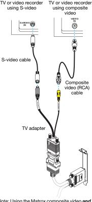
(Note: Using the Matrox composite video and S-video connectors at the same time is optional.)
