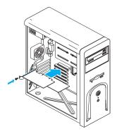
Your Matrox card is now installed. *Before restarting your computer*, connect your monitor or monitors ("Connection setup", page 7). *After connecting*, restart your computer and install your Matrox software (see "Software setup", page 11).
