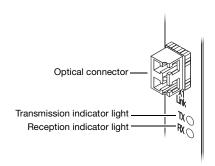
If the transmission indicator is red, your optical connector may be loose. Make sure your optical connector is firmly in place by pushing it into its housing. If the light doesn't change to green, contact your Matrox representative.
