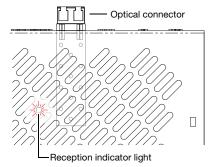
Cause Your optical cable may be defective. Solution Change your optical cable.
