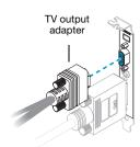
If your Matrox card has 2 DVI connectors, use a DVI-to-HD15 adapter to connect the TV output adapter to the secondary DVI connector (B) of your graphics card.
