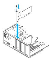
Your Matrox card is now installed. *Before restarting your computer*, connect your monitor or monitors (see "Connection setup", page 6). *After connecting*, restart your computer and install your Matrox software (see "Software installation", page 11).
