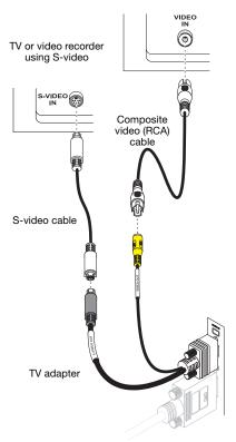
(Note: Using the Matrox composite video and S-video connectors at the same time is optional.)
