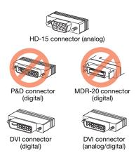
Some monitors with DVI connectors support both digital and analog input. If you're using one of these monitors with your Matrox product, make sure it's configured to use the correct type of input. For more information, see your monitor documentation.
