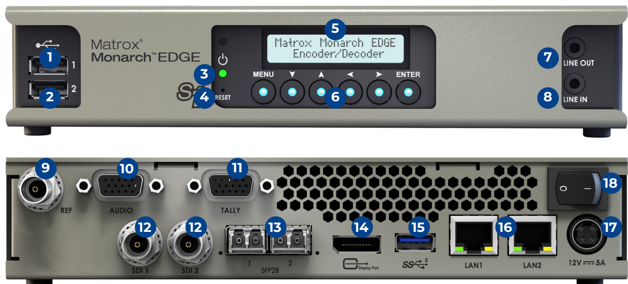
Matrox Monarch EDGE (encoder/decoder connections)
