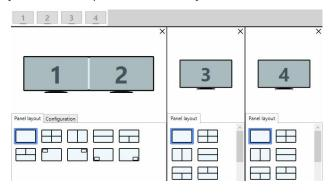
**4** For a layout with joined monitors, from the Configuration tab, select a monitor layout option from Monitor position and set the bezel value(s). Note: For a 1 x 4 configuration, you can set only the horizontal bezel value in Horizontal bezel (pixel). For a 4 x 1 configuration, you can set only the vertical bezel value in Vertical bezel (pixel). For a 2 x 2 configuration, you can set both the horizontal and vertical bezel values.
