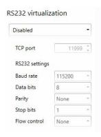
RS232 settings can be done for multiple devices simultaneously using the Multi-device settings option. For more information, see "7.9 - Modify settings", page 96.
