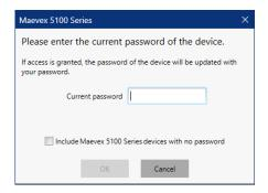
2 Enter the existing password for the device in the Current password field and click OK. The device password is updated with your environment password.
