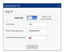
4 Enter your user name in the User name field, the password in the Enter device password field, reenter the password in the Confirm device password field, then click Apply.
