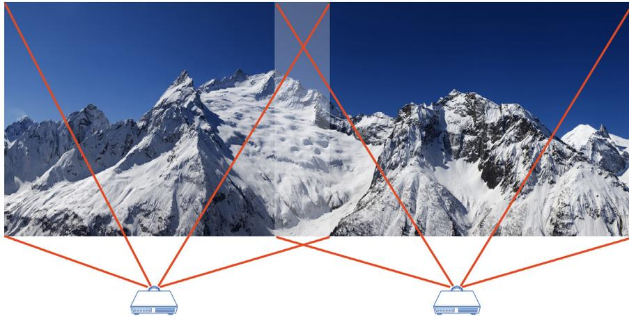
Overlapped image with no edge-blending support makes the projected image blurry and appear brighter along the cross-hatched area.
