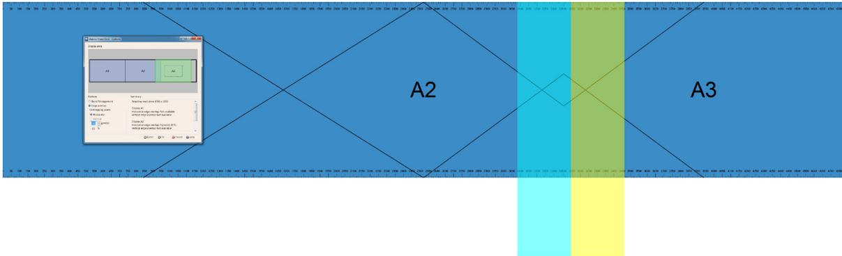
In the illustration above, the area under the light blue and green rectangular bands represents the overlapped area in the UI grid. Using these tools, the user can simply and effectively manage the overlap area to adjust the number of overlapping pixels between the projectors to flawlessly display a single seamless image across three edge-blending projectors.
