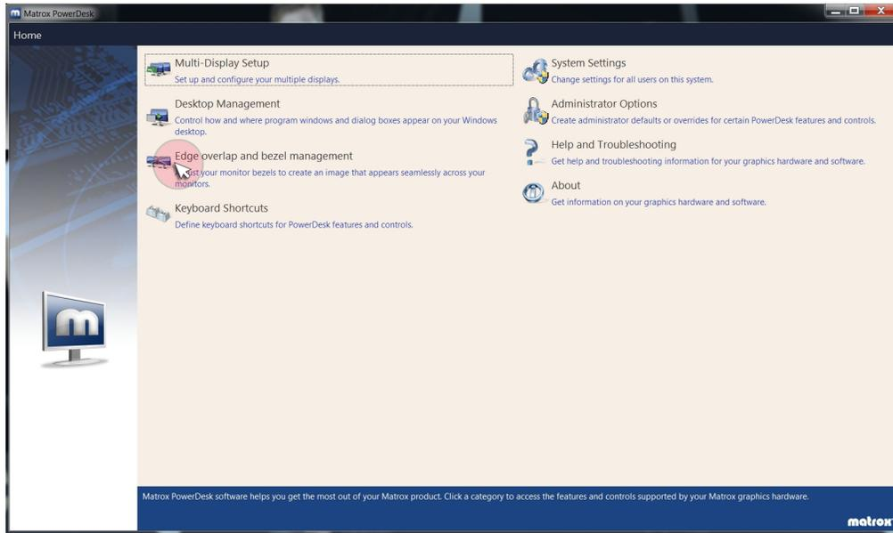
3. Select “Edge Overlap” and adjust each projector horizontal and/or vertical seams by choosing the overlap pixel density.
