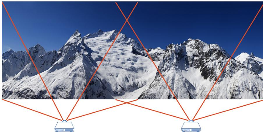
Edge Overlap creates a precisely aligned, unified image across multiple edge-blending projectors. The result is a perfectly blended and seamless image.
