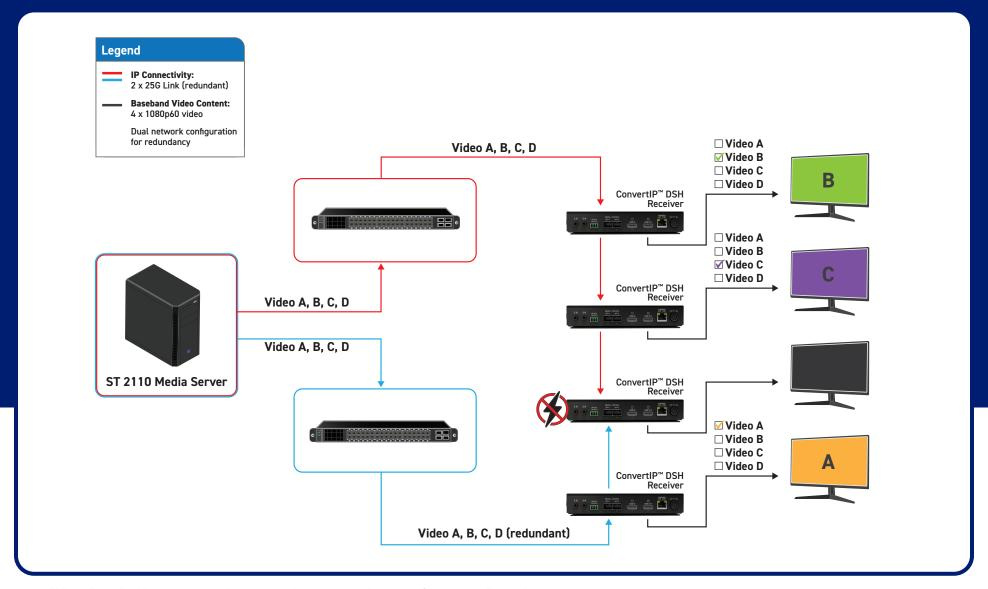
When Installed in 2022-7 environment, view content in case of a power disruption.
