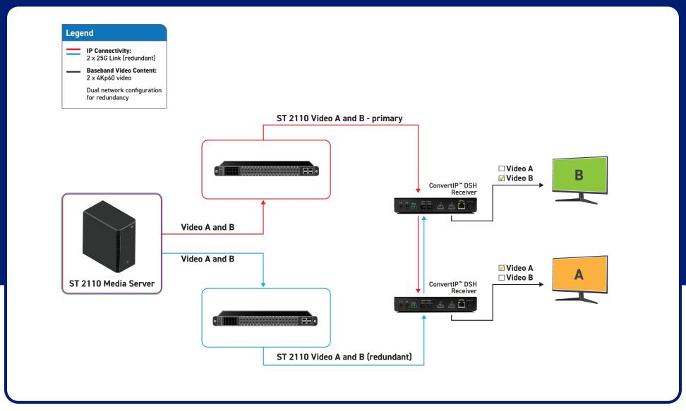
ConvertIP receivers configured in Daisy-chain mode converting UHD 2110 video content [2160p59.94] for HDMI monitoring.
