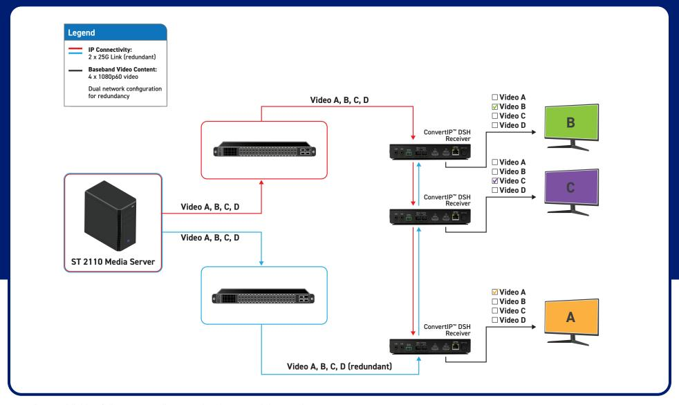
Re-establishing full 2022-7 easily route signals to remaining monitors.
