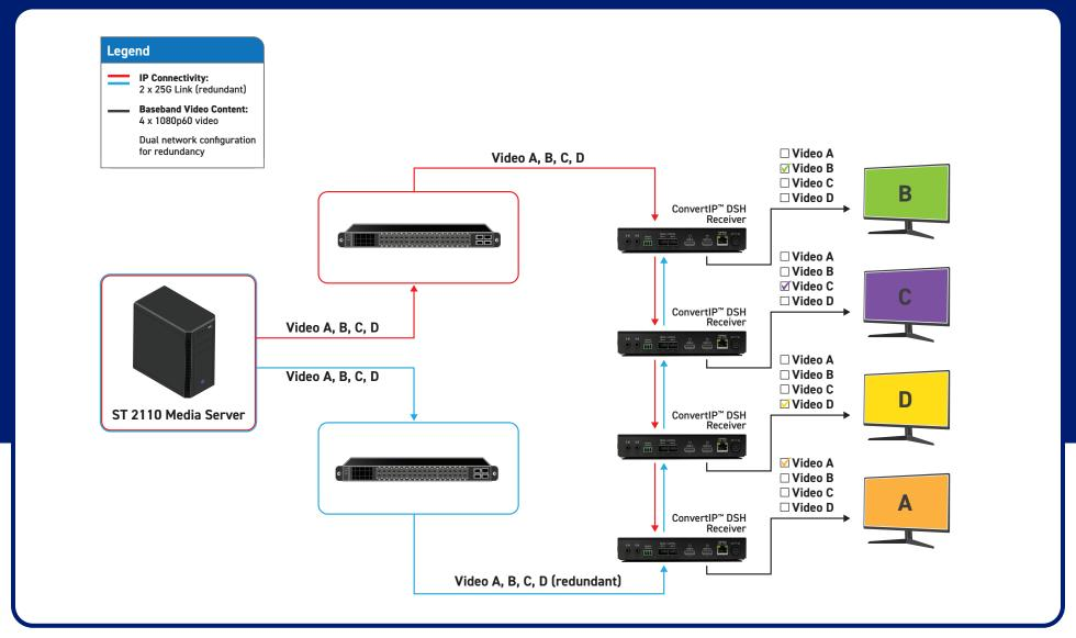
ConvertIP receivers configured in Daisy-chain mode converting FHD 2110 video content [1080p59.94] for HDMI monitoring.
