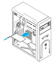
Your Matrox card is now installed. Before restarting your computer, connect your monitor or monitors ("Connection setup", page 6). After connecting, restart your computer and install your Matrox software (see "Software setup", page 8)
