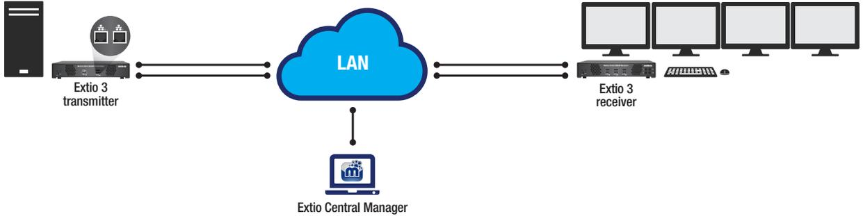
Extio 3 transmitter and receiver appliances can be configured to support redundant network interfaces
