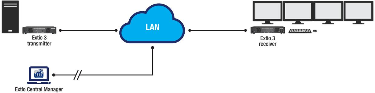
Extio 3 IP KVM's distributed model of operation eliminates single point of failure
