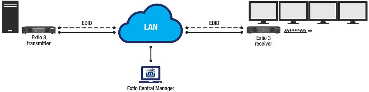
Extio 3's EDID management feature saves monitor's EDID information in the transmitter unit and facilitates seamless operation
